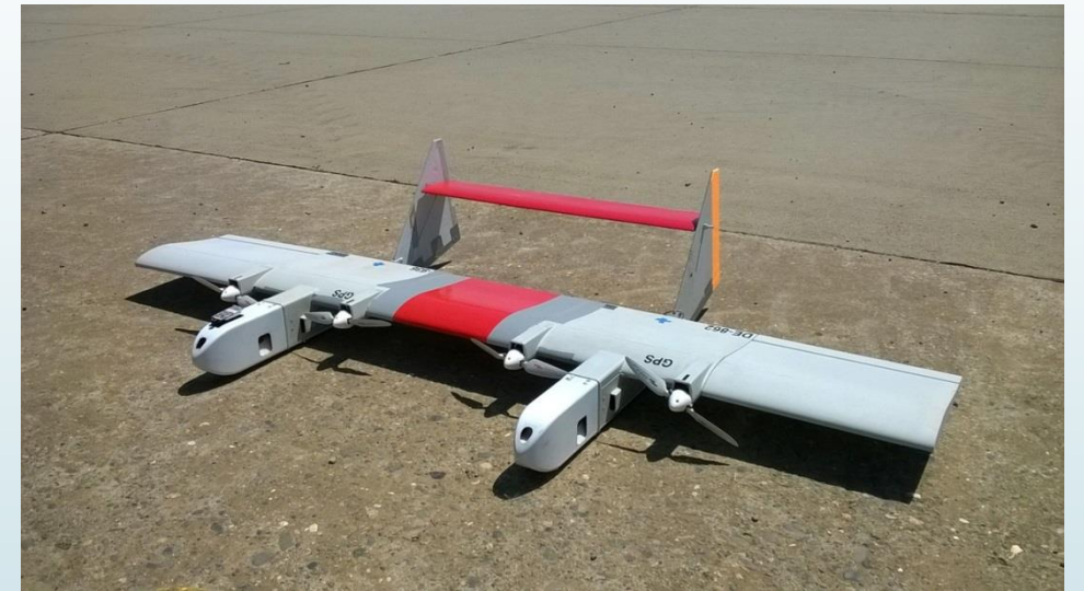
Military surplus RQ-14 DragonEye UAVs dismantled for parts and reassembled into new "FrankenEye" aircraft.
